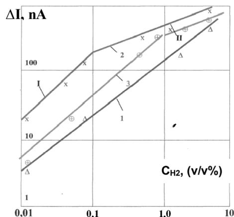
Fig.3. Hydrogen sensor with fluorine-conducting  $\text{Pb-Sn/Pb}_{0,9} \text{Al}_{0,05} \text{Ti}_{0,05} \text{F}_{2,1}$  electrolyte/indicator electrode:
