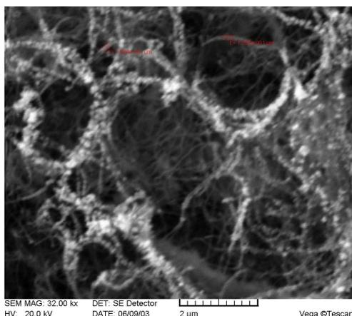
Fig.1. A transverse chip of the sample. From the bottom there are TiN and MWNT moiety layers above which there is a thin layer composed of nanofibers.
