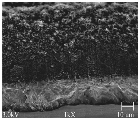
Fig.2. The view of the sample from the above. Amorphous Pd clusters cover the nanofibers surface.
