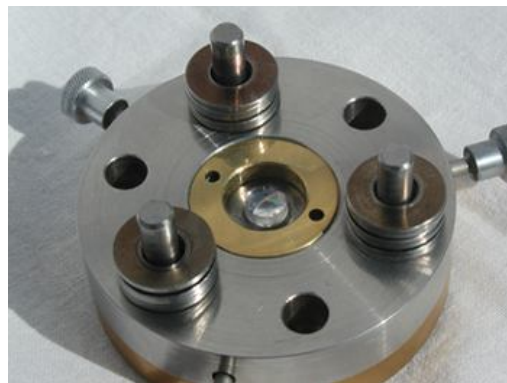
Fig. 1. The high pressure chamber with sapphire anvils ( P=10 GPa, \varepsilon=10^4 W/cm 2 ).
