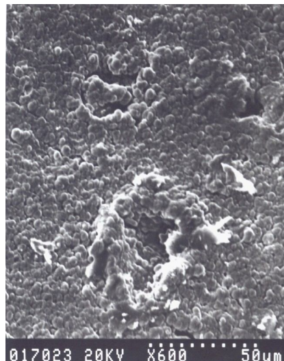
Photo 2. SEM of Ni/ \alpha -Al 2 O 3 membrane. Top surface of nickel coating obtained by magnetron sputtering.
