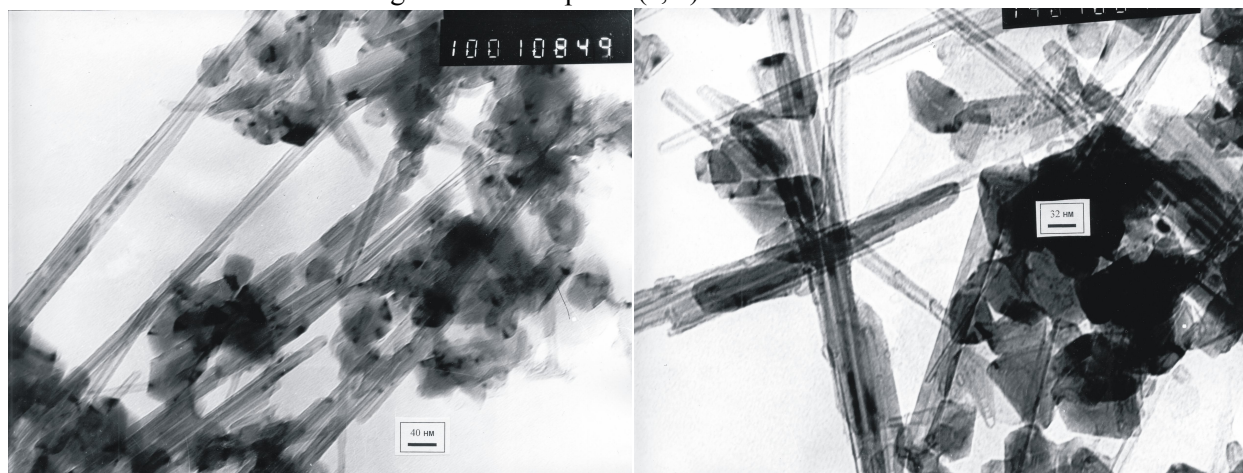
Fig.2. Core of deposit. (a, b) Bunches of nanotubes
